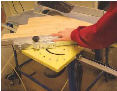
▲ Pic.4 Use the table saw to trim the top and bottom panels to shape and size, then clean up both faces using planes and scrapers
